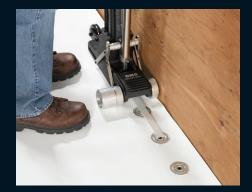
AccuSeam has a measuring tail for accurate spacing and removable wheel extensions for walls and curbs.
