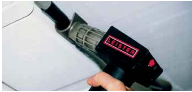
Shrinking cable connections with the GHIBLI.
