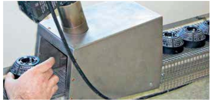
The HOTWIND hot air blower is perfectly-suited for drying and baking of print onto plastic components.
